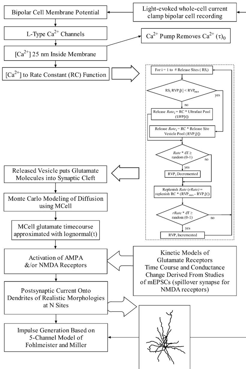
Fig. 1. A flow diagram of the program elements in the ribbon synapse model.
